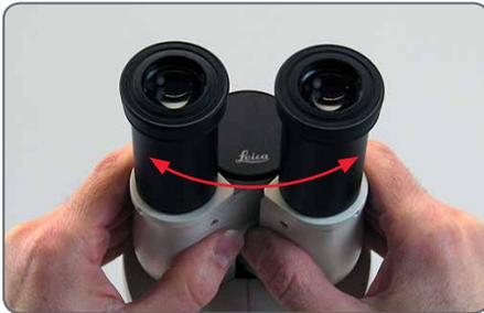
**i** The length of the tubes remains the same for all pupillary distances. This means that a change in pupillary distance has no effect on parfocality, magnification or magnification-dependent calibrations.
